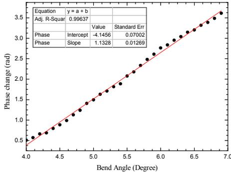
Figure 4 Interferometric phase change versus inclinometer rotation angle.
