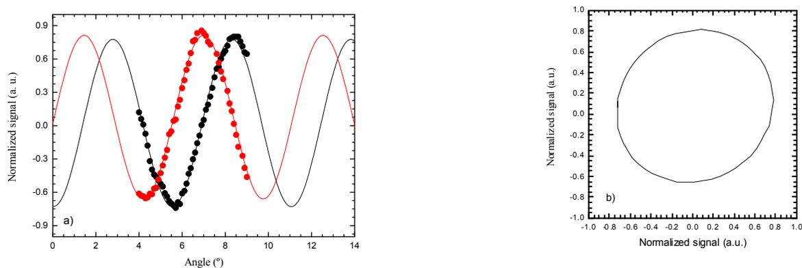
Figure 3 (a) Photodetected signals versus inclinometer bend angle (dots: experimental measurements, lines: fitting curve), and (b)  $x$ - $y$  signal representation illustrating the quadrature condition.
