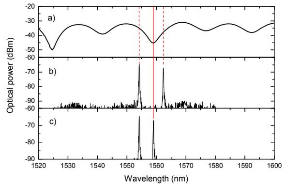
Figure 2 Spectral responses of (a) the fibre-taper-modal Michelson interferometer, and (b) the fibre Bragg gratings. (c) The spectral quadrature position.
