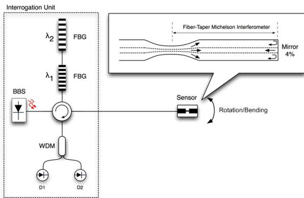
Figure 1. Experimental set-up for the optical interrogation of the proposed fibre inclinometer. Inset: schematic diagram detail of the fibre-taper-modal Michelson interferometer.
