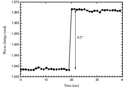
Figure 5 Inclinometer sensor resolution (measurement bandwidth: 1 Hz).
