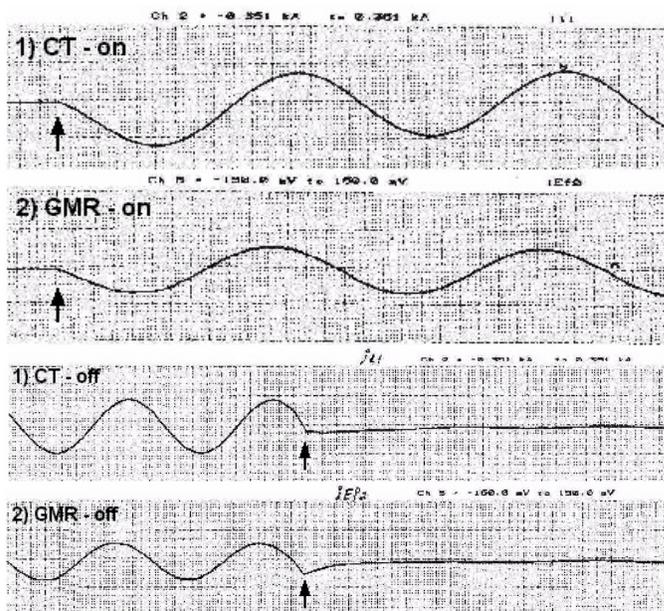
Fig. 4 Relaying field test of 310  $A_{\text{RMS}}$  current signal at 50 Hz on a 150 kV high voltage power line (CT – conventional current transformer, GMR – optoelectronic current transformer).
