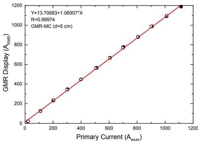
Fig. 3 Output response linearity of the optoelectronic current transformer to applied primary current at 50 Hz frequency.
