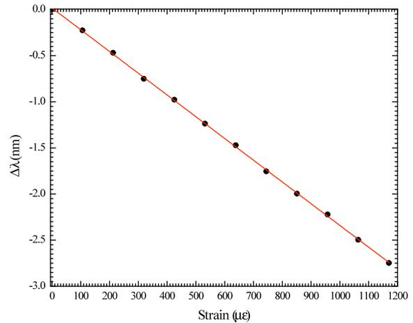
Figure 3 - Strain response of the sensing head.
