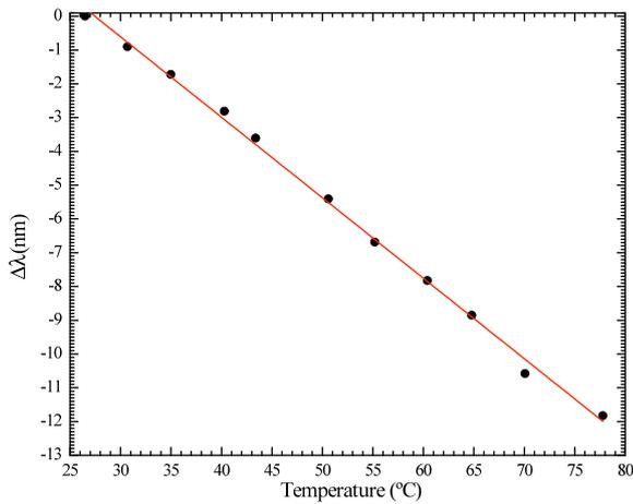
Figure 4 - Temperature response of the sensing head.
