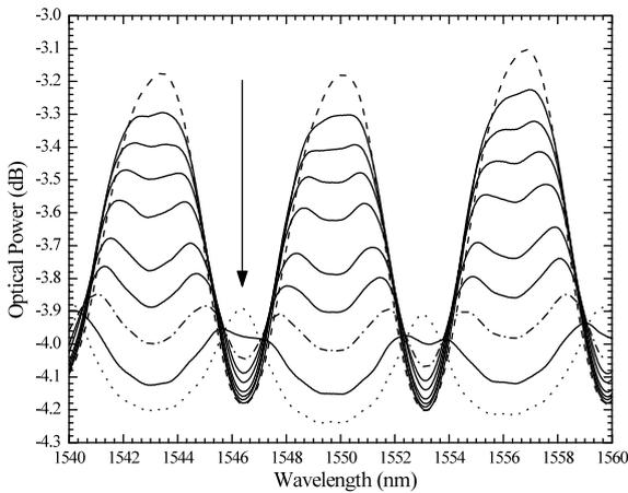
Figure 2 - Channeled spectrum of the sensing configuration when one paddle of the polarization controller was moved.
