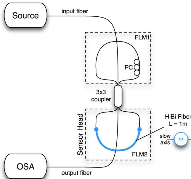
Figure 1 - Schematic of the experimental setup, exhibiting the cross-section of the HiBi fiber used.
