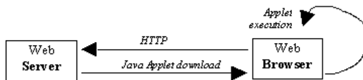
Figure 12: the Applet is executed in the client side
