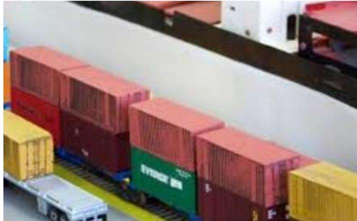
Figura 7.43 — Transporte *double stack*.
