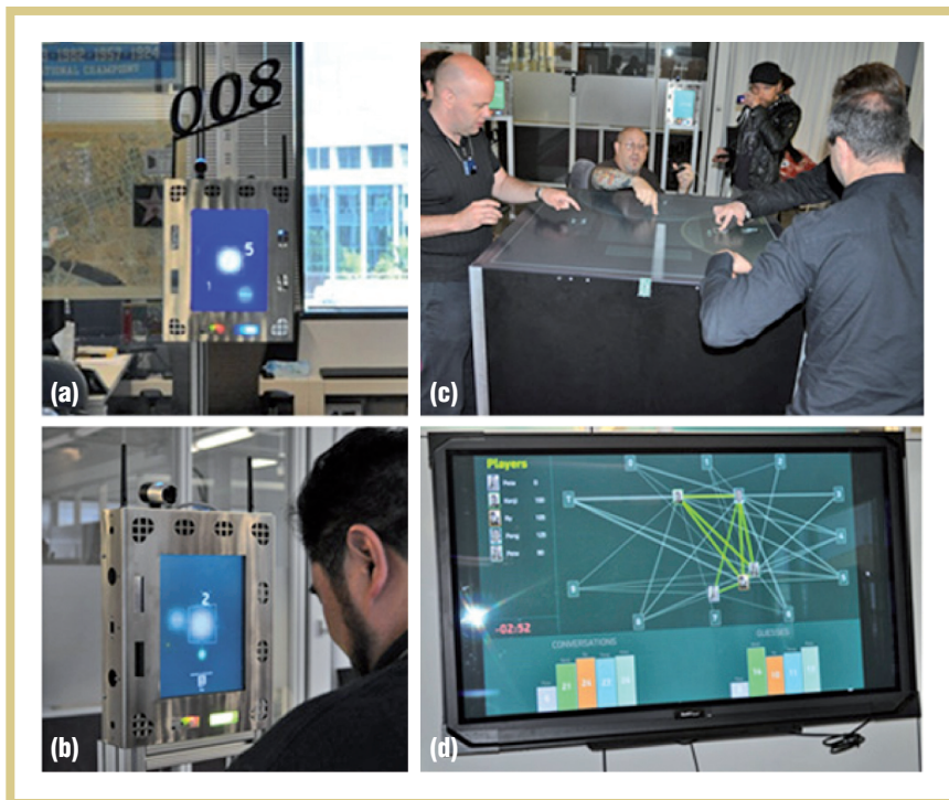
Figure 2. The platform’s portal and interactive table. (a) Mirror #008 mounted on a strut and hanging from the ceiling, (b) the badged user interacting with a mirror, (c) the multitouch, multiuser BrickTable in collaborative use, and (d) a status display showing overall game status and social connection data.
