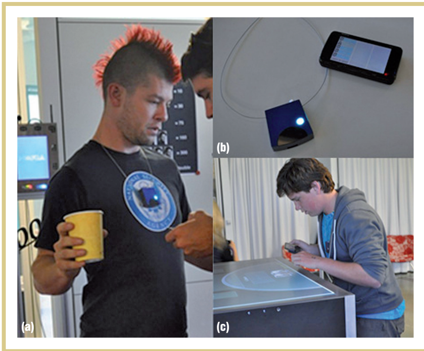
Figure 1. The badge for the pervasive computing platform. (a) A user wearing the badge, (b) a badge paired with a mobile device using Bluetooth, and (c) a user wearing the badge and using a multitouch table for collaborative actions while simultaneously using the mobile device for private actions. The badge lets both work with the user’s specific data.
